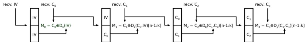
Shift register de  $n$  bits,  $k = n / 2$ ;  $C_i, M_i$   $n / 2$  bits
